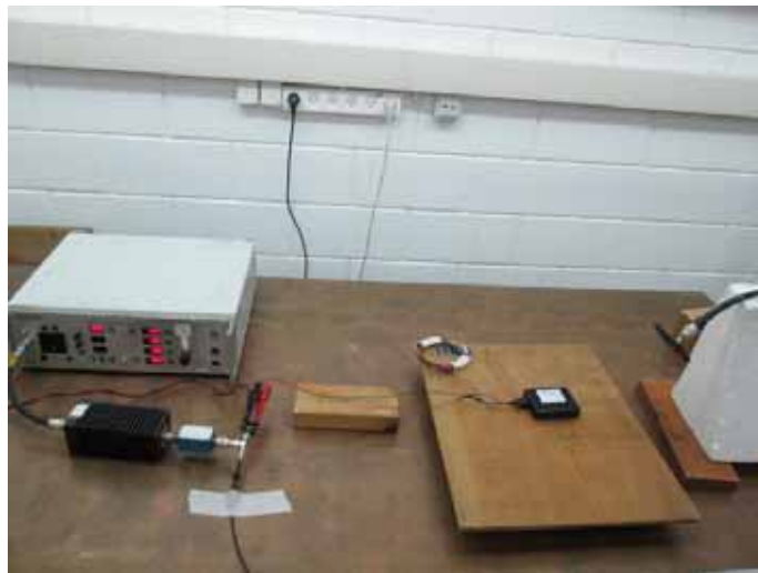
Photograph 8.3.8 Conducted transients on power line test setup, Pulse 3a and Pulse 3b
