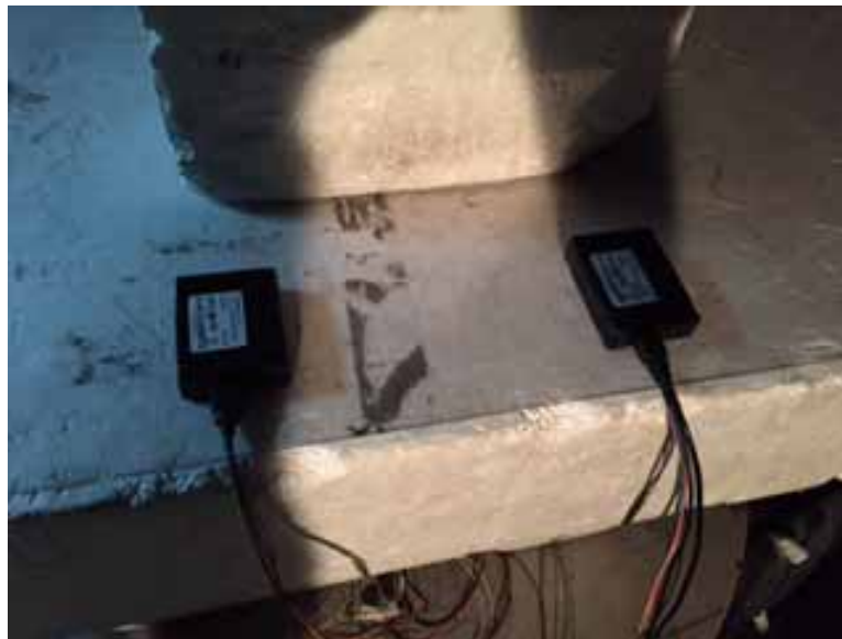
Photograph 7.3.2 Setup for radiated emission measurements, EUT cabling, CR300B 2G, part number CT7801201-000 & CR300B 3G EU, part number CT7801202-000 together
