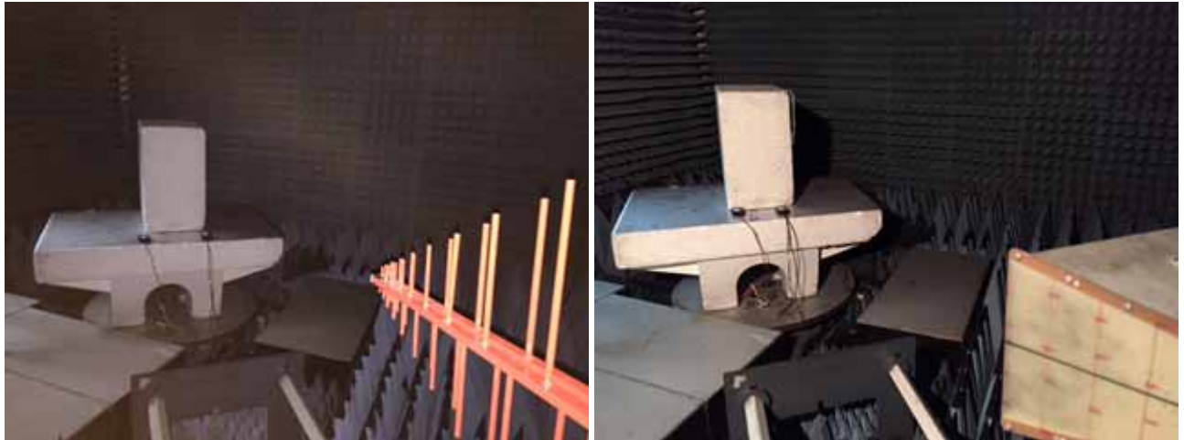
Photograph 7.3.2 Setup for radiated emission measurements, EUT cabling, CR300B 2G, part number CT7801201-000 & CR300B 3G EU, part number CT7801202-000 together
