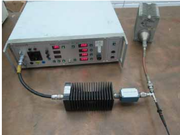
Photograph 8.3.7 Conducted transients on power line calibration setup, Pulse 3a and Pulse 3b
