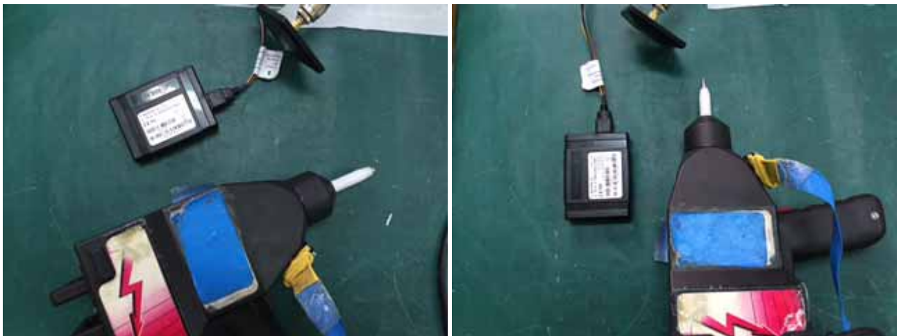
Photograph 8.1.1 Setup for immunity to ESD, general view
