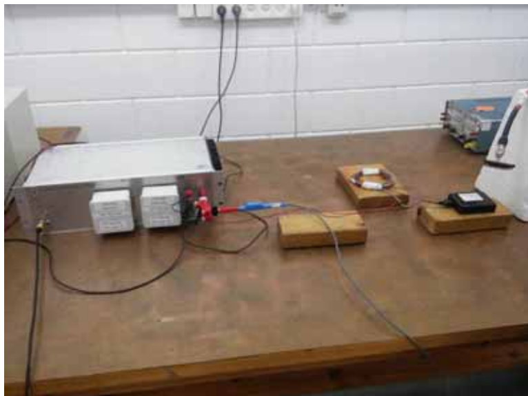
Photograph 8.3.4 Conducted transients on power line test setup, Pulse 2a
